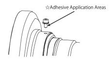
Caution: Please apply an adhesive (i.e. ThreeBond 1401 or equivalent) on thread ( $\not \simeq$ ) when using it while wearing it.
