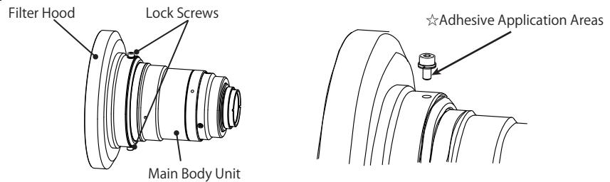
Caution: Please apply an adhesive (i.e. Threebond 1401 or equivalent) on thread (☆) when using it while wearing it.
